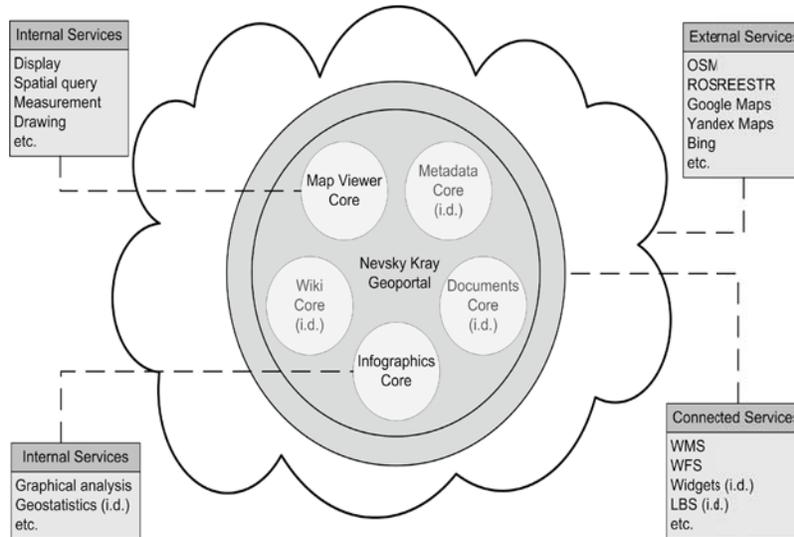
Fig.2. Services configuration of the Nevsky Kray Geoportal (i.d. means 'in development').
