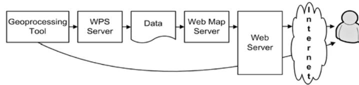
Fig.4. Hybrid model of geoprocessing Web-services.
